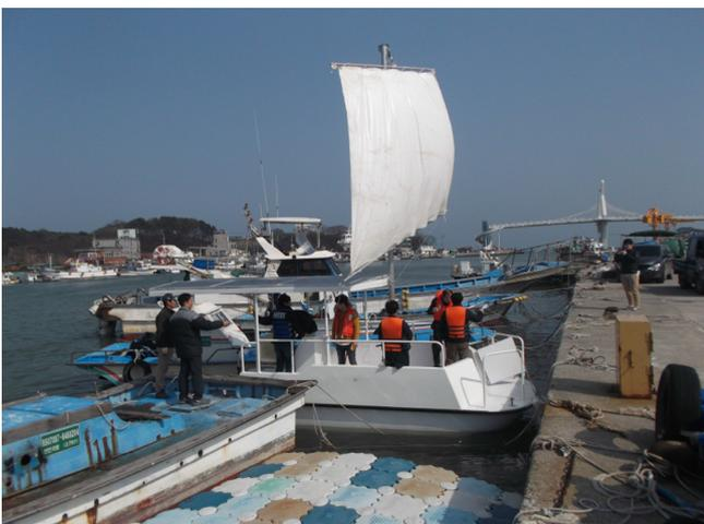
Fig. 10 Image to show the manufactured prototype of eco-environmental leisure ship with wind and solar energy
