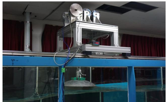
Fig. 5 1:20 scale WEC model on basin
