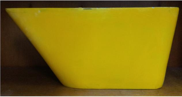
Fig. 2 Stabilizer fin for model experiment
