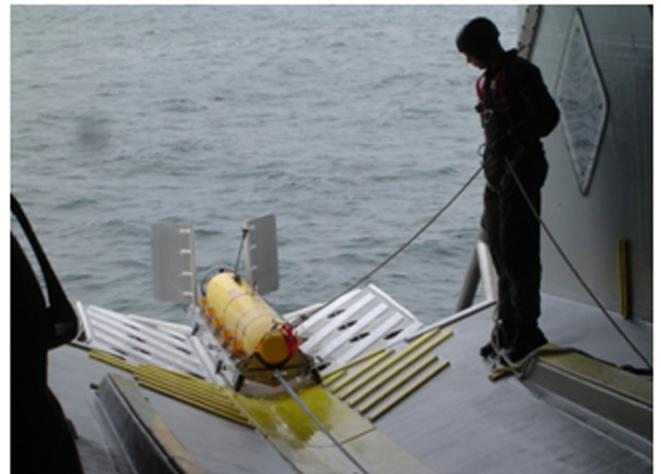
Fig. 4 UUV storage and launch concept in M80 Stiletto (Mship C., 2015)
