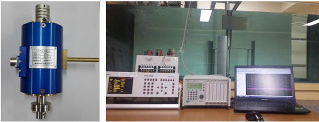
Fig. 13 Torquemeter and measuring equipments
