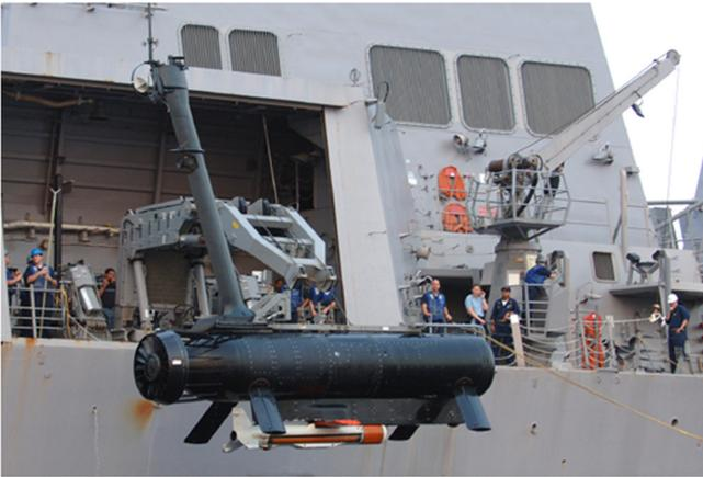
Fig. 2 RMS UUV launch from USS Monsen by A-frame type davit system (Lockheed Martin Co., 2016)
