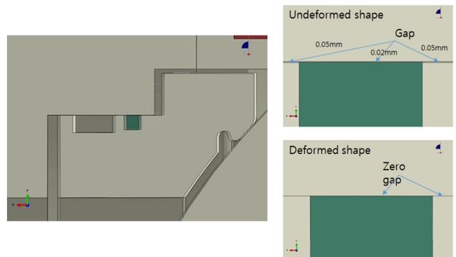
Fig. 18 Deformation with graphite
