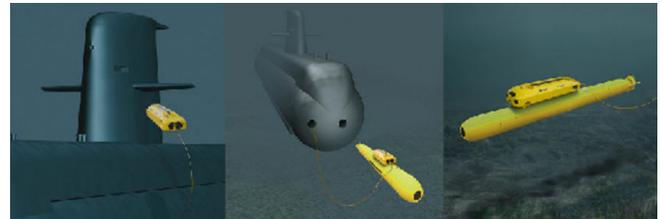
Fig. 13 Sea Owl SUBROV launch and recovery concept (Saab Seaeye Ltd., 2015)
