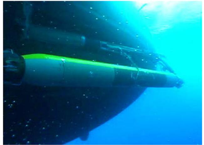
Fig. 12 Robot arm LMRS UUV recovery system (White, 2007)
