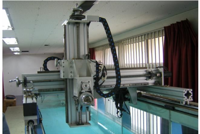
Fig. 4 Forced oscillation device
