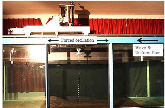
Fig. 7 Slender body model test in regular waves
