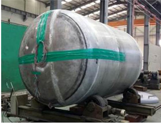
(a) Adhesion of strain gage on inner tank
