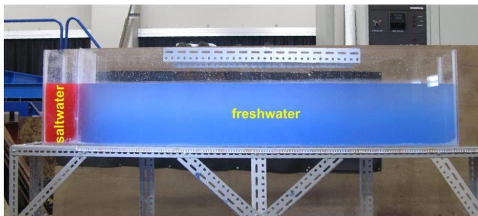
Fig. 2 Setup of water basins for laboratory experiments
