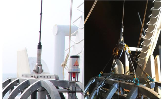
Fig. 2 1-point Hinge connection (left), 4-point wire connections (right)
