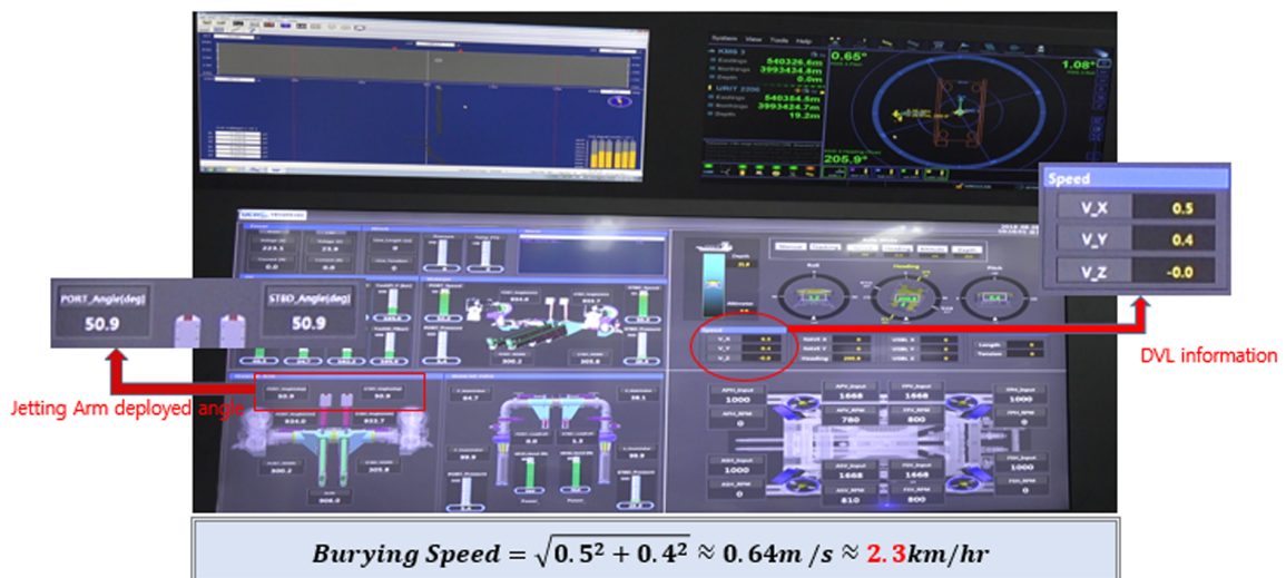
Fig. 19 Sea trial result: burying speed
