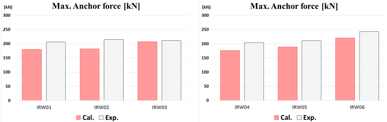
Fig. 12 Comparisons of maximum anchor force (left: wave only, right: combined environment)
