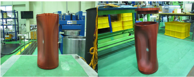
Fig. 5 Collapse of thick aluminum cylinder (Choi et al., 2016)
