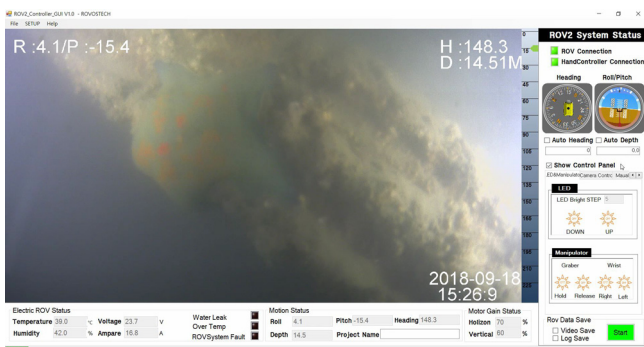
Fig. 10 Captured image of outside border displayed in pilot console
