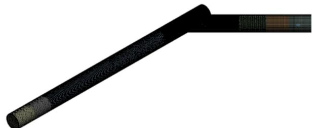
Fig. 13 Grid of capped wye ( $\theta = 45^\circ$ )
