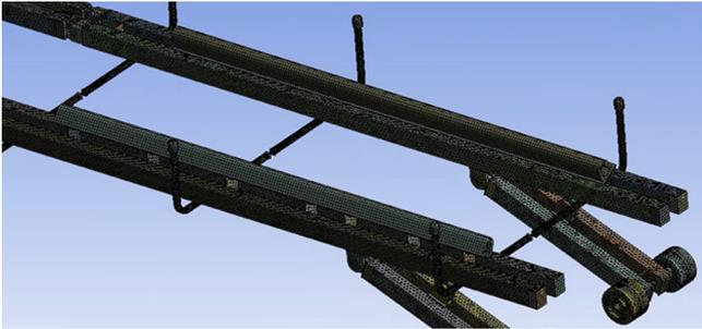
Fig. 6 Finite element mesh of transporter
