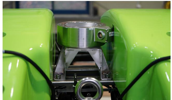
**Fig. 6** F/T (Force/Torque) sensor fixed on ROV
