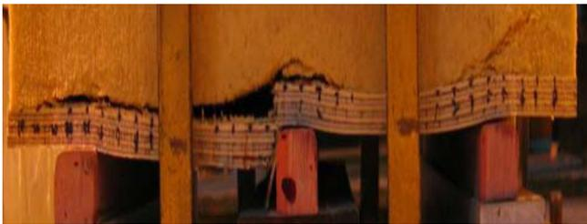
Fig. 2 Shear fracture of plywood in Mark-III type
