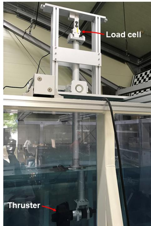
Fig. 2 Experimental equipment for measuring thrusting force
