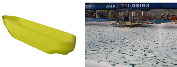
Fig. 1 Hull shape of the Arctic FPSO used in the experiment and simulation and overall environment of the model test in progress
