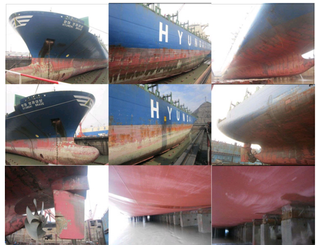
(a) Before blasting & painting
