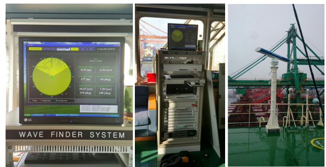
Fig. 6 Photographs of wave radar on 8,600 TEU container ship
